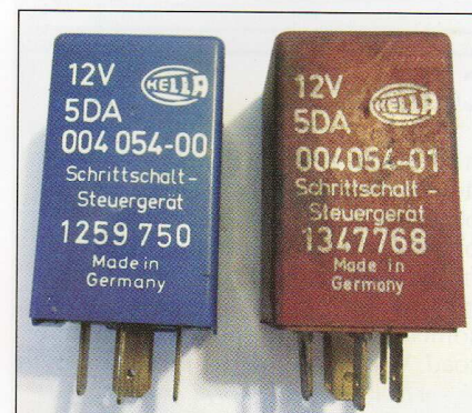
Blue relay, part 1259750, and Volvos from 1985-1993 used a Red one, part 1347768.
