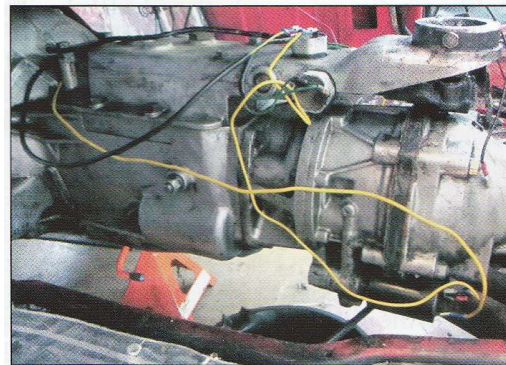
Wiring at the overdrive unit, it won't be this easy on a MGB.
