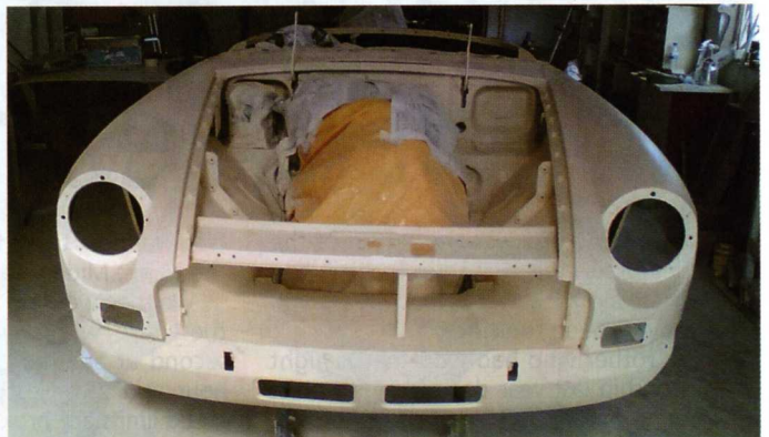
The shell stripped and resprayed
