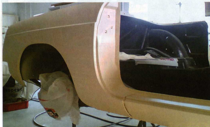
The shell stripped and resprayed
